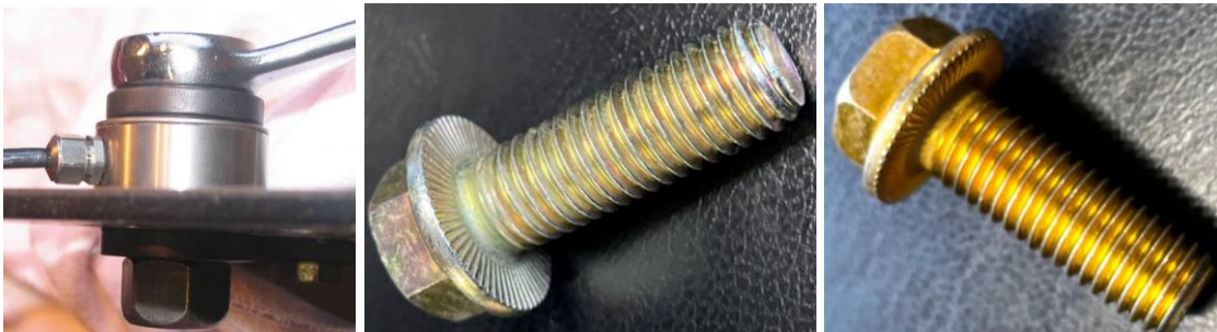
Figure 5 – Change of bolt supplier projects, generally allowed provided preload is not degraded and backed up with preload testing.
