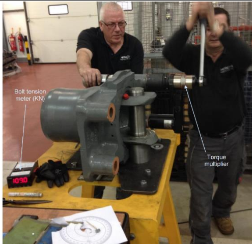
Figure 6 – Bolt reuse projects. Allowed providing torque tightening is replaced with angle tightening procedure.
