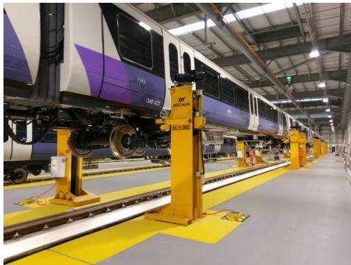
Figure 8 – Train lift accident investigation due to screw jack wear and deficiency in safety nut design as dynamic loading not accounted for. Bonus: insurance case reports and structural repair of permanently deformed bodyshell.
